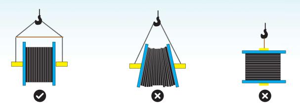
When manipulating with the drums using a crane, a spacer rod has to be placed between the load bearing ropes, so that the ropes do not exert pressure on the cable through the side drums.
