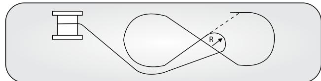
**Note:** R Minimum Permissible bending radius of cable.
